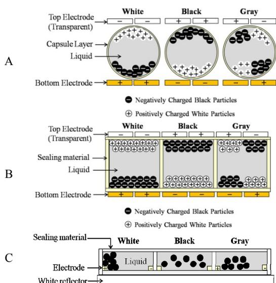
**Fig. 4.** (A) E-ink microcapsules electrophoretic display structure and working principle; (B) Microcup electrophoretic display structure and working principle; (C) In-plane electrophoretic display structure and working principle.
