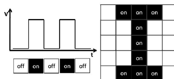
**Fig. 1.** Schematic drawing of the digital display principle. Left: top is the curve of driving signal and bottom is the sketch of frontplane material showing white and black fluids driven by signal to switch on and off, respectively. Right: a letter “I” is shown in black by switching on the corresponding pixels or segments.
