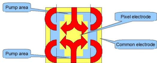
**Fig. 5.** Schematic pixel geometry of EOD. (Copyright from ref.<sup>61</sup> with permission from SPIE).
