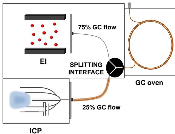
Accurate quantitation and characterization of organometals is successfully achieved by splitting the GC flow to both an electron ionization mass spectrometer (EIMS) and an inductively coupled plasma mass spectrometer (ICPMS).
