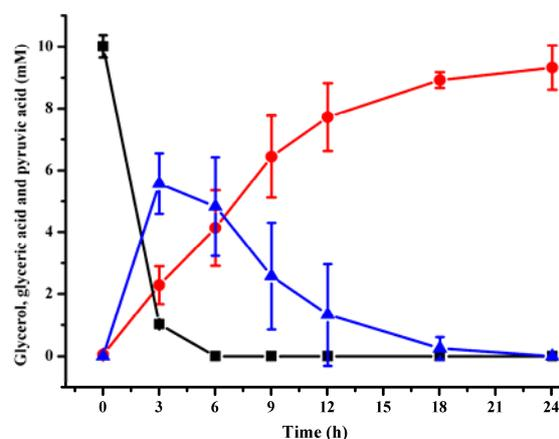
**Fig. 3.** Conversion of glycerol into pyruvic acid by the artificial reaction cascade. Glycerol (■), glyceric acid (▲), pyruvic acid (●). The reaction was carried out in a 100 mL screw-capped bottle with 30 mL of reaction broth containing 100 mM HEPES buffer (pH 7.4), 10 mM glycerol, 0.3 U mL<sup>-1</sup> Aldo, 0.1 U mL<sup>-1</sup> DHAD, and 1000 U mL<sup>-1</sup> catalase. The reaction was conducted at 50°C and a shaking speed of 300 rpm. Results are means ± SD of three parallel replicates.
