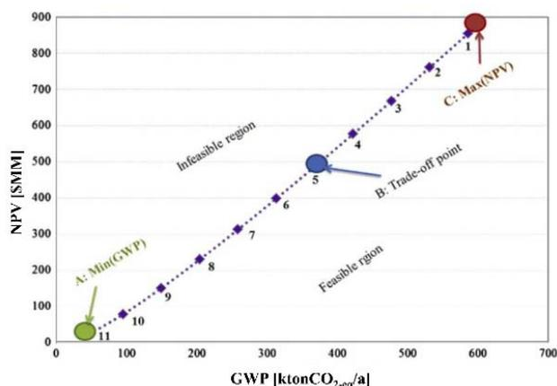
Figure 16: Pareto optimal curve for a hydrocarbon bio refinery<sup>64</sup> reprinted with permission from Elsevier.
