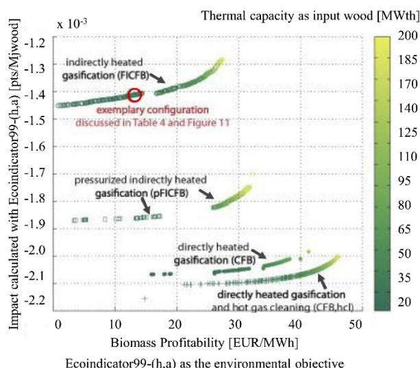
Figure 15: Results of multi-objective optimisation using the Eco-Indicator 99 impact as the environmental objective, biomass profitability as the economic objective, at multiple scale<sup>113</sup> reprinted with permission from Elsevier.
