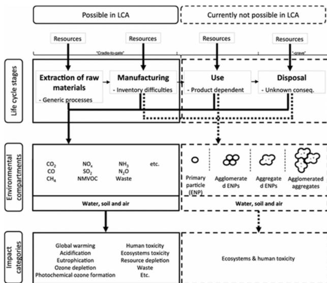
Figure 19: Limitations of LCA of engineered nanomaterials, according to Miseljic *et al.*<sup>123</sup> with kind permission from Springer Science and Business Media.
