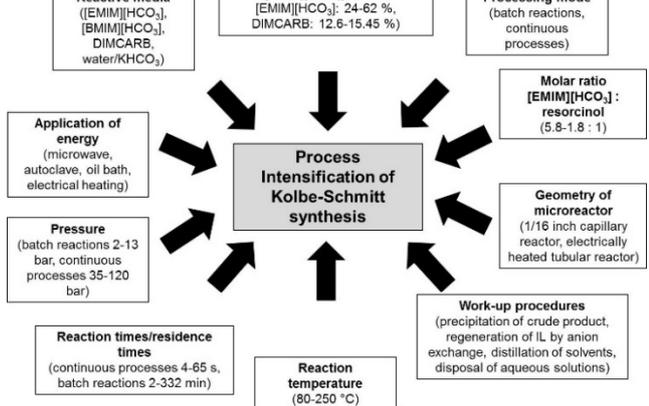
Fig. 14: Concepts for PI of Kolbe-Schmitt synthesis by Kressirer *et al.*<sup>30</sup> reprinted with permission from the American Chemical Society.
