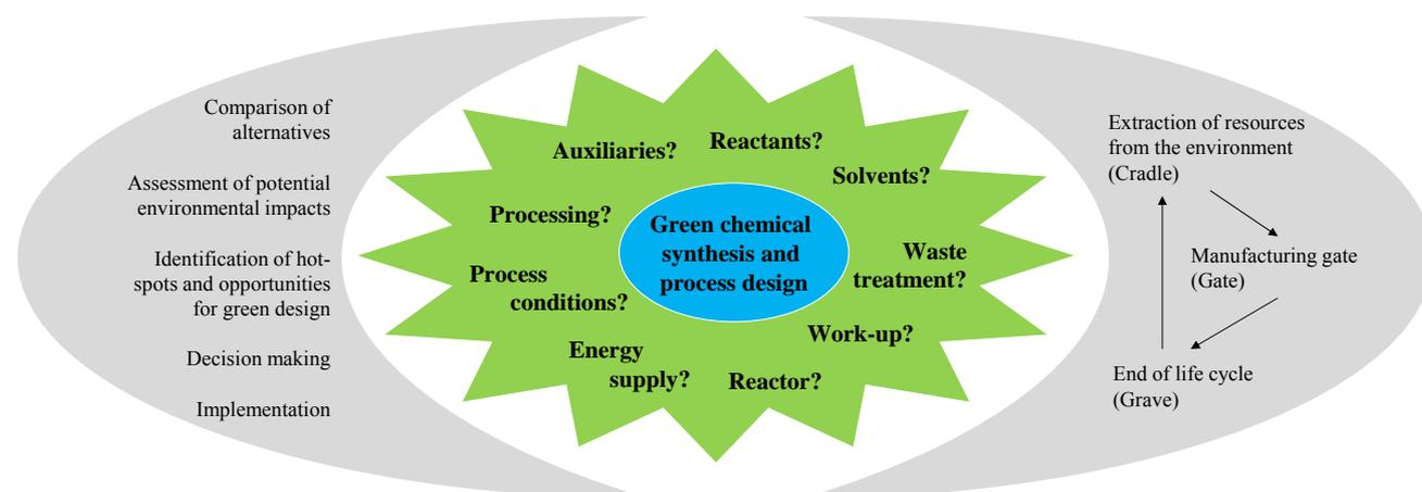
Figure 1. Life-cycle thinking in green chemical synthesis and process design.
