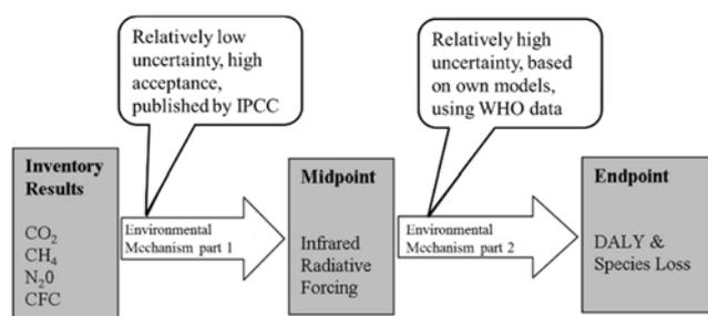
Figure 3. Illustration of a harmonised midpoint-endpoint model for climate change, linking to human health and ecosystem damage applied within ReCiPe.<sup>10</sup>
