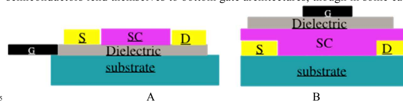
Figure 3 A “Bottom gate” and B “Top gate” OFET architectures. D, drain; G, gate; S, source; SC, semiconductor.
