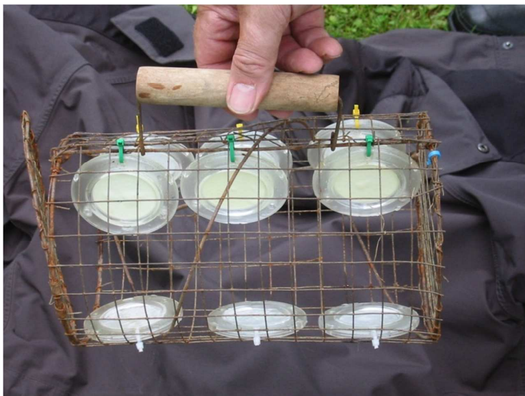
Fig. 1. Typical deployment of Chemcatcher passive sampler in the natural water.
