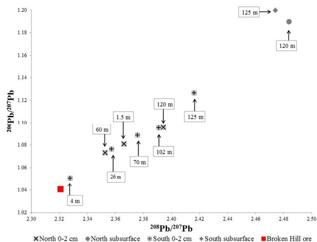
**Figure 4:** Soil lead isotopic compositions at either side of the rail line at Triple Chance, benchmarked against Broken Hill ore.
