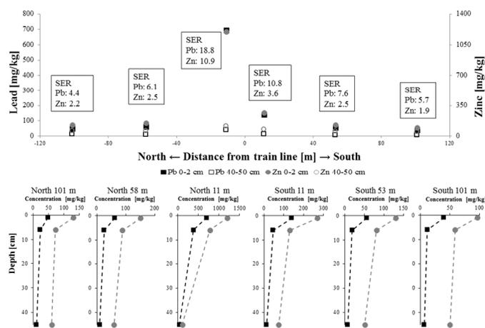
**Figure 2:** Soil lead and zinc soil concentration profiles either side of Silverton train line.
