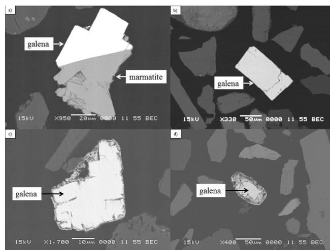
**Figure 5:** SEM micrographs of dust samples (scales shown on images) a) House #1 ~40-80 $\mu\text{m}$  composite crystalline galena and marmatite particle. b) House #2 ~150x 75 $\mu\text{m}$  galena particle. c) Galena particle from House #2. d) Galena particle from House #2.
