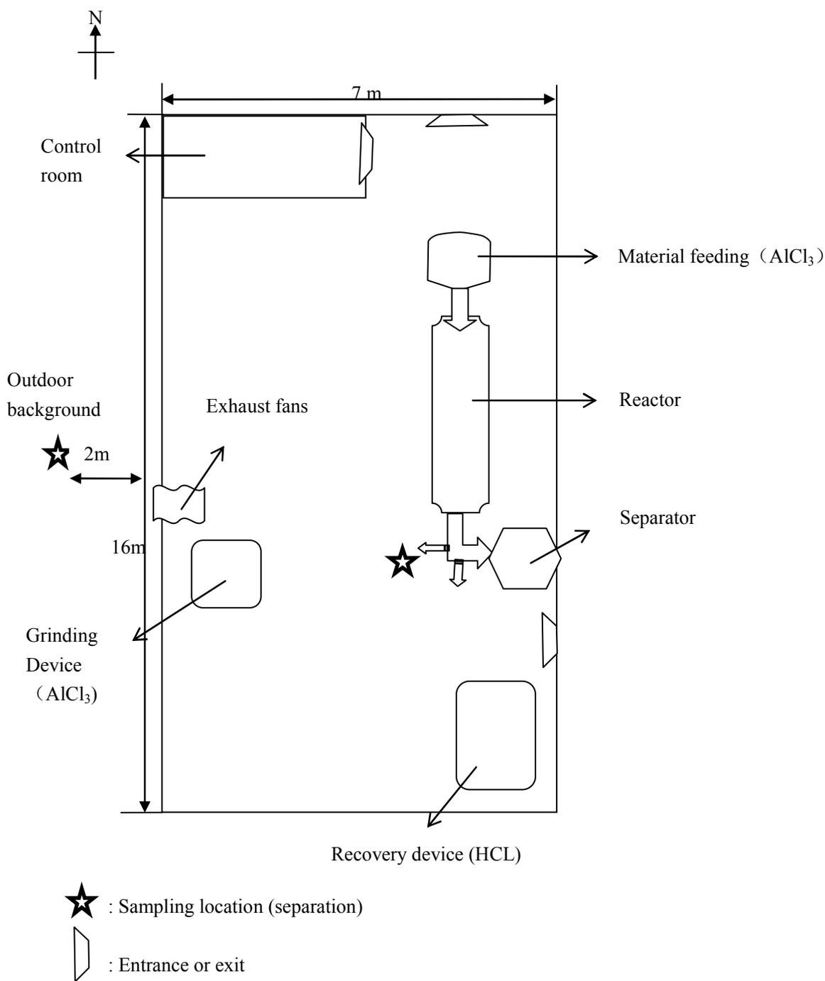
Fig.1 (a) Production workshop layout and sampling location
