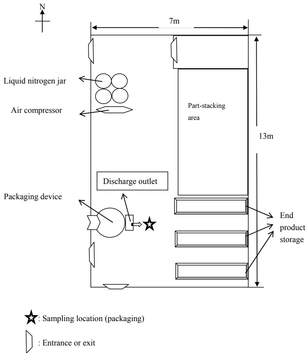
Fig.1 (b) Packaging workshop layout and sampling location
