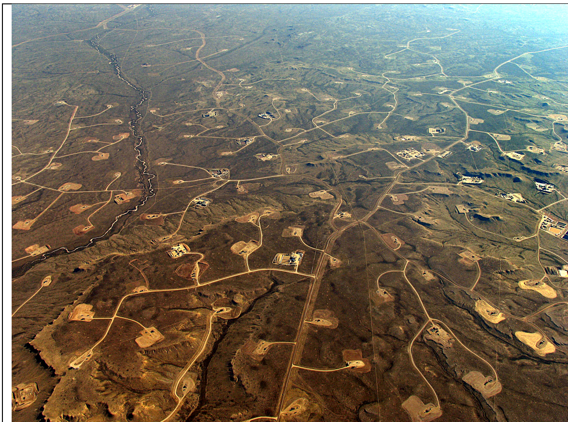
Fig. 5 The Jonah Field development in the Upper Green River Basin, Sublette County, Wyoming is expected to produce gas for up to 50 years from 1,500 wells. Photo courtesy of Skytruth.
