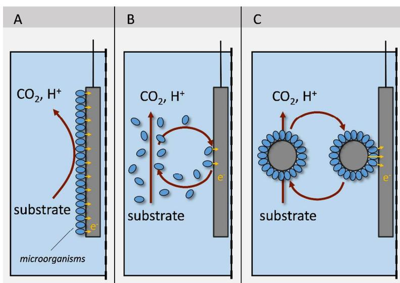
**Figure 4:** Direct electron transfer in exemplary anodic BES half-cells A) Biofilm electrode, B) via suspended cells, C) via capacitive biofilm particles
