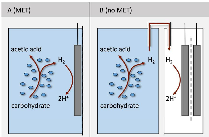
**Figure 6:** A) Anodic half-cell of a hydrogen-mediated BES B) Hybrid system consisting of a fermenter and a separate hydrogen fuel cell.
