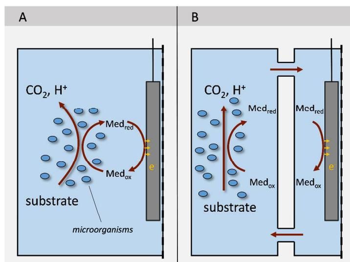
**Figure 5:** Mediated electron transfer in exemplary anodic BES half-cells A) Integrated ("conventional") BES, B) BES consisting of separate fermenter and electrochemical cell.
