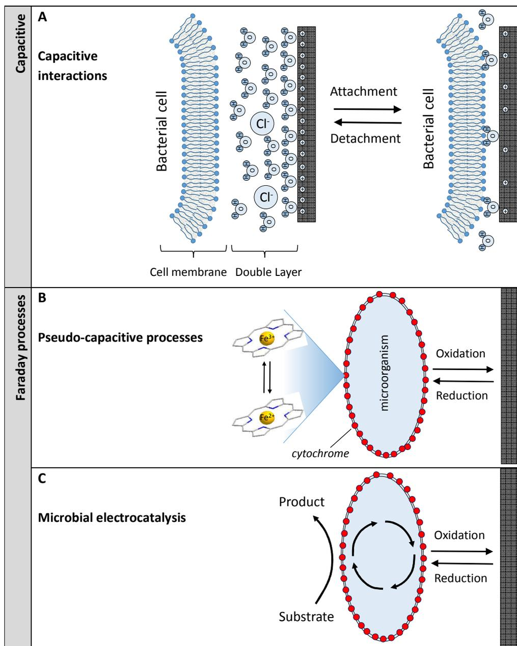
**Figure 2:** Major electrochemical interactions between microorganisms and electrodes.
