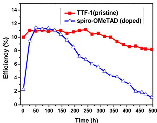
**Fig. 4** Efficiency variation of optimized cells based on dopant-free TTF-1 (pristine) and p-type doping spiro-OMeTAD (doped). Unencapsulated cells were stored in air at room temperature with a humidity of about 40% and were measured under illumination at AM 1.5 G.
