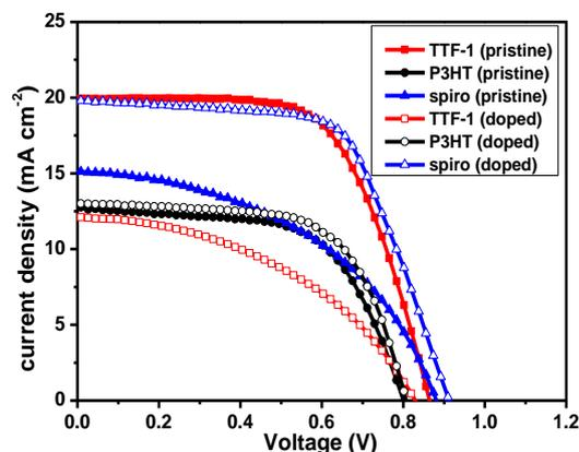
Fig. 3 Current–voltage curves of typical small-area (0.09 cm<sup>2</sup>) perovskite solar cells based on TTF-1, P3HT, and spiro-OMeTAD in their pristine form or doped with Li-TFSI and TBP, respectively.
