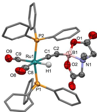
**Fig. 4** Molecular structure of **4** with 50% probability displacement ellipsoids. For clarity, most hydrogen atoms have been omitted and phenyl groups simplified. Selected bond distances [Å] and angles [°]: Ru1–C1 2.060(7), Ru1–H1 1.560, Ru1–C8 1.899(8), Ru1–C9 1.955(8), C1–C2 1.21(1), B1–C2 1.54(1), B1–N1 1.666(9), Ru1–C1–C2 178.1(6), C1–C2–B2 171.5(8).
