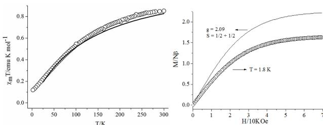
**Figure 6.** Temperature dependence of  $\chi_{\text{M}}T$  (left, the solid line represents the best fit based on the parameters discussed in the text) and Field dependence of magnetization at 2 K of complex **3** (right). The calculated curves are based on  $S_{\text{Fe}} = 1/2$ ,  $S_{\text{Cu}} = 1/2$  and  $g = 2.09$ .
