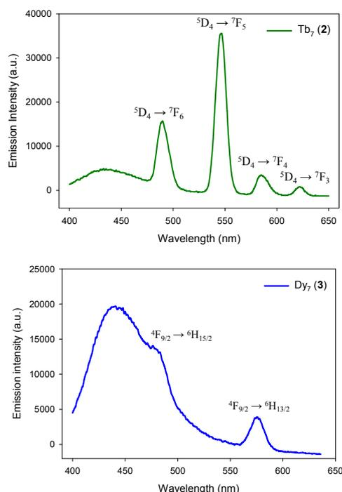
**Fig. 4** Room temperature emission spectra for **2** (top) and **3** (bottom) in MeCN (10<sup>-5</sup> M). The excitation wavelength was 340 nm in both cases.
