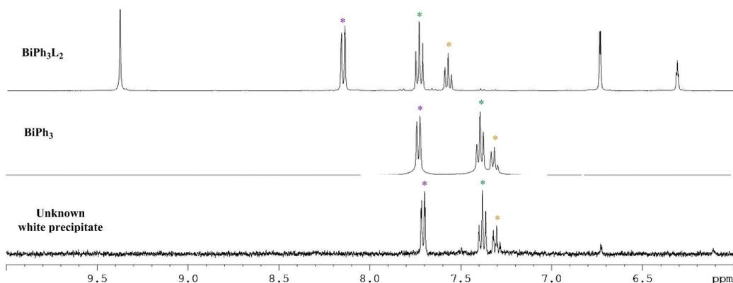
**Figure 4.**  $^1H$  NMR spectra of **2B**,  $BiPh_3$  and unknown white precipitate in  $d_6$ -DMSO at 25°C.
