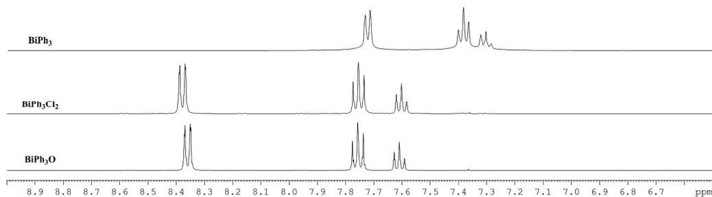
**Figure 5.** Comparison of the <sup>1</sup>H NMR spectra of [BiPh<sub>3</sub>O], BiPh<sub>3</sub> and starting material [BiPh<sub>3</sub>Cl<sub>2</sub>] in d<sub>6</sub>-DMSO at 25°C.
