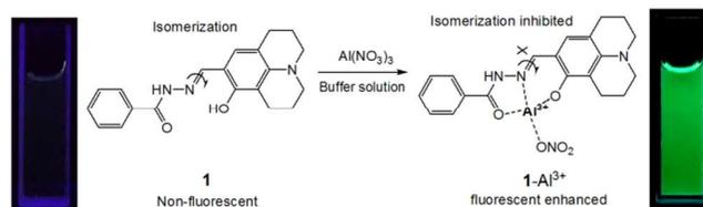
Scheme 2 Fluorescent enhancement mechanism of **1-Al<sup>3+</sup>** complex.
