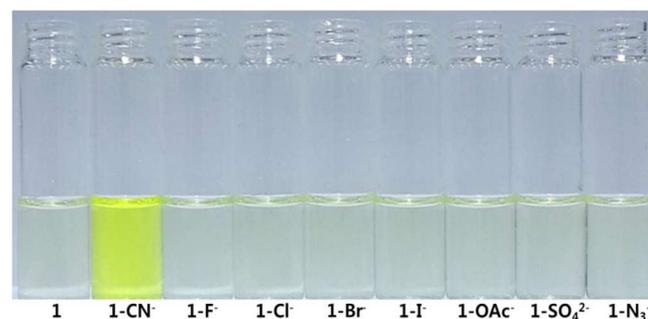
Fig. 9 (a) Absorption spectra changes of **1** (30  $\mu\text{M}$ ) in the presence of 200 equiv of different anions (b) The color changes of **1** (30  $\mu\text{M}$ ) upon addition of various anions (200 equiv) in bis-tris buffer/methanol (7/3, v/v).
