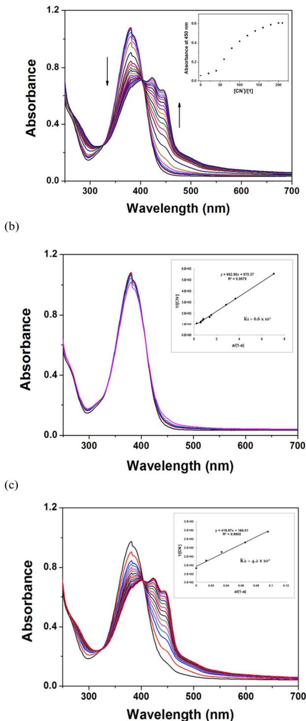
**Fig. 10** (a) Absorption spectra changes of **1** (30  $\mu$ M) after addition of increasing amounts of CN<sup>-</sup> (10, 20, 30, 40, 50, 60, 70, 80, 90, 100, 110, 120, 130, 140, 150, 160, 170, 180, 190 and 200 equiv) in 10 mM bis-tris buffer/methanol (7/3, v/v) at room temperature. Inset: Absorbance at 450 nm versus the number of equiv of
