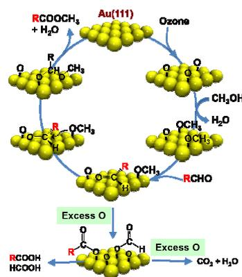
**Scheme 1** Schematic of reaction mechanism for aldehyde coupling with methanol on the oxygen-covered Au(111) surface.<sup>7</sup>
