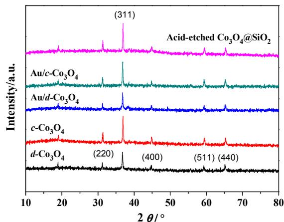
**Fig. 4** XRD patterns of various Co<sub>3</sub>O<sub>4</sub>-based catalysts.
