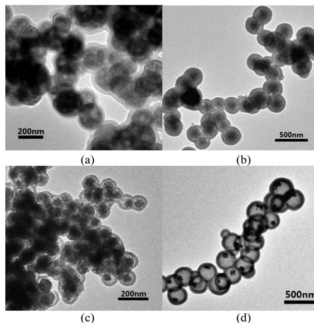
**Fig. 3** TEM images: (a) non-acid-etched Co<sub>3</sub>O<sub>4</sub>@SiO<sub>2</sub>, (b) slightly acid-etched Co<sub>3</sub>O<sub>4</sub>@SiO<sub>2</sub>, (c) moderately acid-etched Co<sub>3</sub>O<sub>4</sub>@SiO<sub>2</sub>, and (d) heavily acid-etched Co<sub>3</sub>O<sub>4</sub>@SiO<sub>2</sub>.
