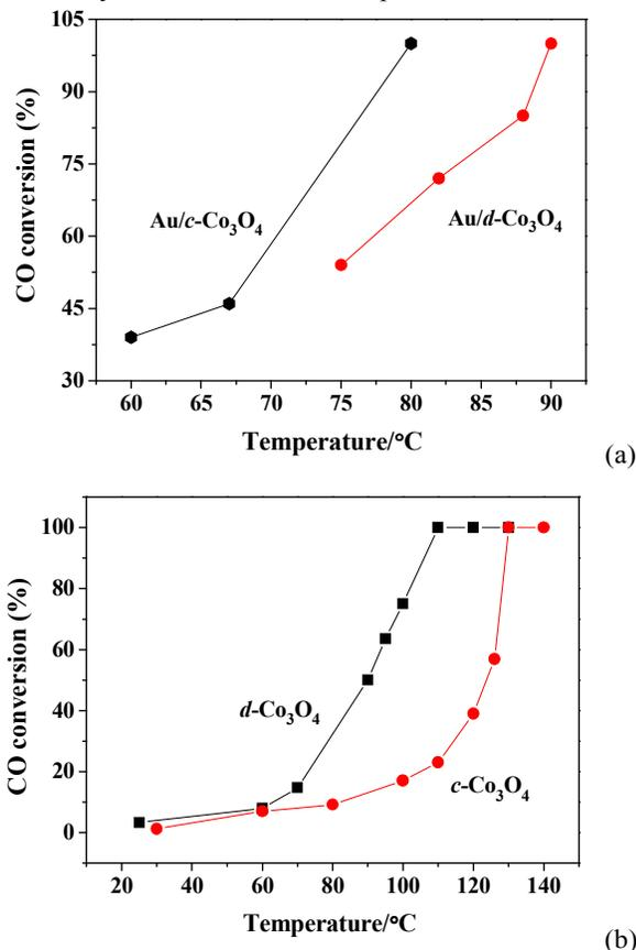
**Fig. 10** Temperature dependence of CO conversion on (a) Au/c-Co<sub>3</sub>O<sub>4</sub> and Au/d-Co<sub>3</sub>O<sub>4</sub> and (b) c-Co<sub>3</sub>O<sub>4</sub> and d-Co<sub>3</sub>O<sub>4</sub>: all of the samples had been subjected to pre-reaction at 350 °C for 5 h.
