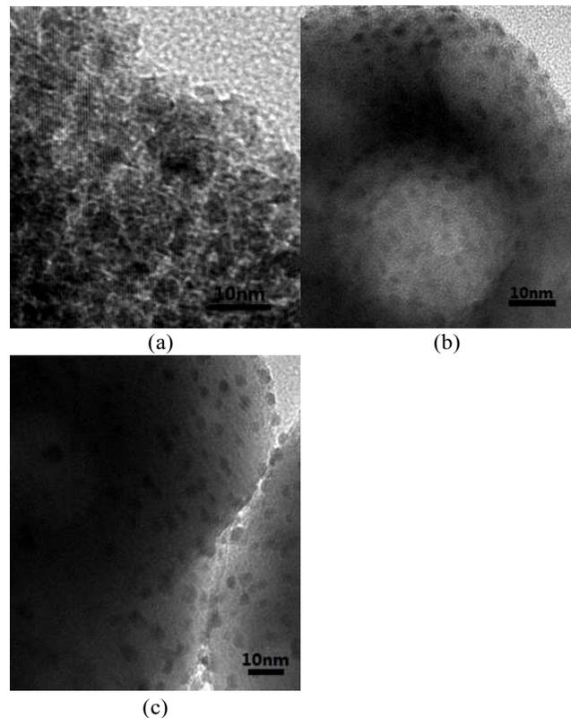
**Fig. 1** TEM images of (a) Au/d-Co<sub>3</sub>O<sub>4</sub>, (b) Au/c-Co<sub>3</sub>O<sub>4</sub>, (c) used Au/c-Co<sub>3</sub>O<sub>4</sub>.
