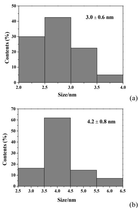
**Fig. 2** Au particle size distribution in (a) Au/c-Co<sub>3</sub>O<sub>4</sub> and (b) used Au/c-Co<sub>3</sub>O<sub>4</sub> (> 70 h reaction).
