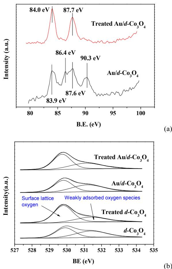
**Fig. 7** (a) Au 4f, and (b) O 1s XPS spectra of the treated and untreated d-Co<sub>3</sub>O<sub>4</sub> and Au/d-Co<sub>3</sub>O<sub>4</sub> nanostructures.
