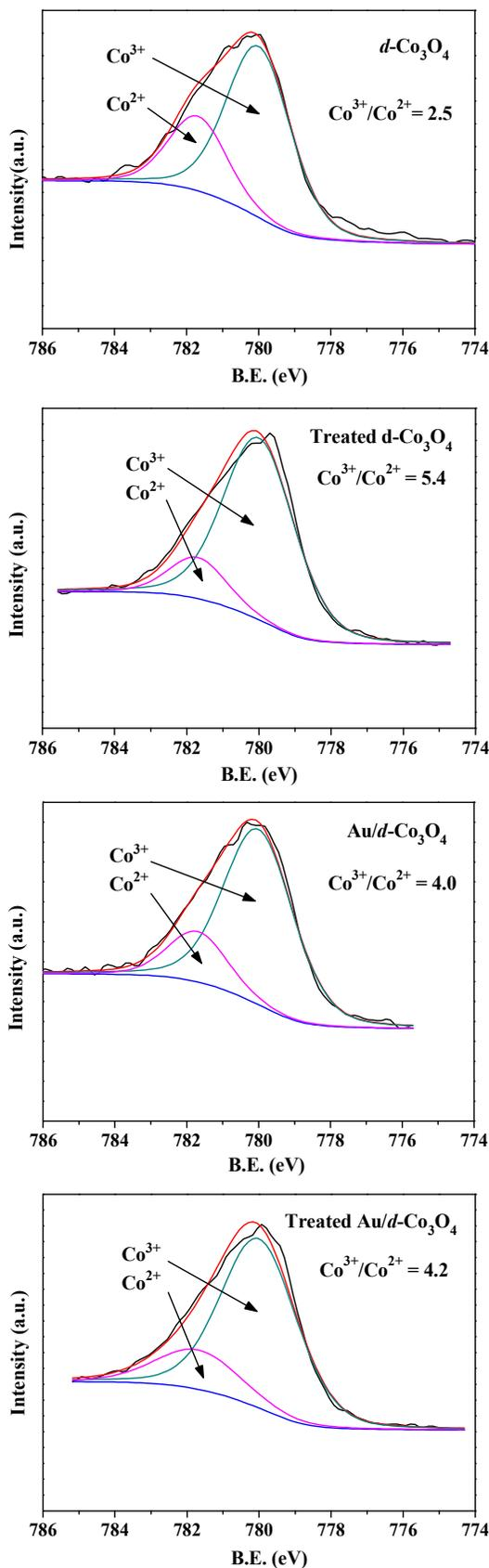
**Fig. 8** Deconvolution analysis of the Co 2p XPS peaks of the untreated and treated  $d\text{-Co}_3\text{O}_4$  and  $\text{Au}/d\text{-Co}_3\text{O}_4$ .
