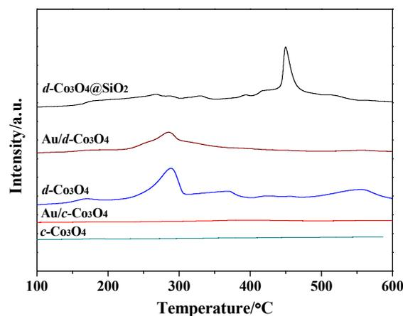
**Fig. 6** O<sub>2</sub>-TPD profiles of the d-Co<sub>3</sub>O<sub>4</sub> and c-Co<sub>3</sub>O<sub>4</sub> based catalysts with and without Au NPs.
