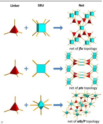
**Fig. 15** Graphic presentation of the topologies associated with MOFs assembled from tetrahedral linkers.
