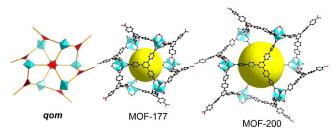
Fig. 11 A qom net shown in augmented form and crystal structures of representative MOFs in its net. Color scheme in qom: Zn<sub>4</sub>O(CO<sub>2</sub>)<sub>6</sub> 5 octahedral cluster (turquoise); tritopic linker (red); color scheme in MOF-177 and 200: zinc (turquoise); O (red); C (black).
