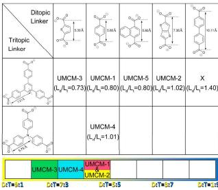
**Fig. 31** The combinations and ratios of tritopic and ditopic linkers used for the preparation of UMCM-1, 2, 3, and 4.
