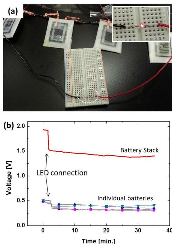
**Figure 3.** (a) Lighting a red LED with the four batteries connected in series (battery stack) and (b) output voltages of the battery stack (solid line) and individual ones when an LED was connected across the four batteries in series.
