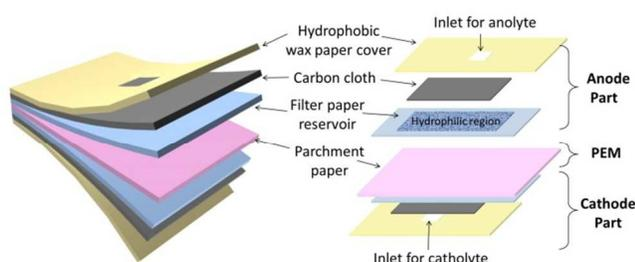
**Figure 2.** Schematic diagram of the paper-based bacteria-powered battery
