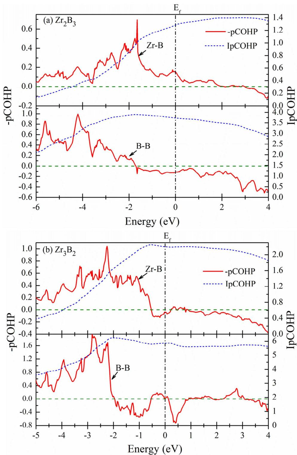
**Fig. 9** Crystal orbital Hamilton population (pCOHP) analyses for the new phases are obtained with the PW/PAW-based method.
