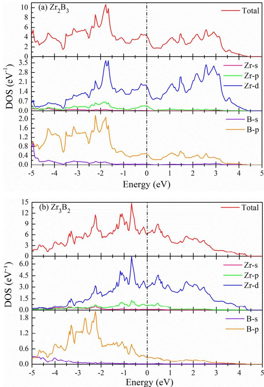
Fig. 7 Partial densities of states for (a)  $Zr_2B_3$  and (b)  $Zr_3B_2$ .
