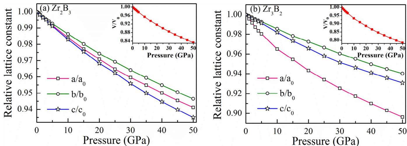
**Fig. 5** Pressure dependence of lattice constants  $a$ ,  $b$  and  $c$  for (a)  $Zr_2B_3$  and (b)  $Zr_3B_2$ . The pressure dependence of cell volume is also shown in the inset.
