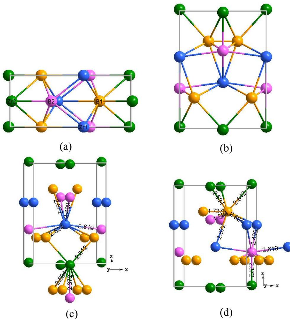
**Fig. 1** Schematic image of  $Zr_2B_3$  is projected along the [100] and [010] directions, respectively [(a) and (b)]; (c) the coordination environment of Zr1 and Zr2 atoms; (d) the coordination environment of B1 and B2 atoms. Zr1, Zr2, B1 and B2 atoms are denoted in blue, green, orange and pink, respectively.
