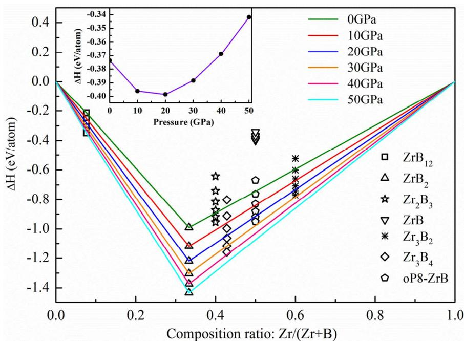
**Fig. 4** The convex hull of Zr-B system at the pressure of 0 ~ 50 GPa. The solid line indicates the convex hull. The enthalpy of formation of ZrB as a function of pressure is also shown in the inset.
