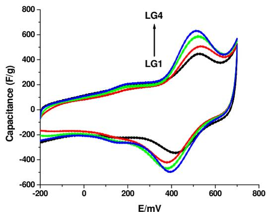
Figure 3. Cyclic voltammograms of the different lignins/PPy composites at 20 mV/s.
