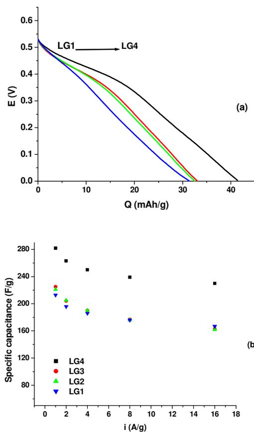
Figure 4. (a). Comparison of the charge capacity of different lignins/PPy composites at 1A/s. (b). Comparison of the specific
