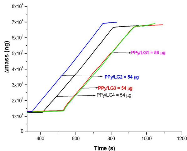
Figure 2. Mass changes obtained for the deposition of the different lignins/PPy composites on gold electrode.
