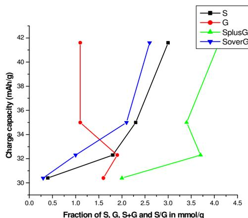
Figure 5. A plot of the variation of the charge capacity against the S(■), G(●), S + G(▲) fractions as well as the S/G ratio(▼) (no units) found in the different lignins studied.
