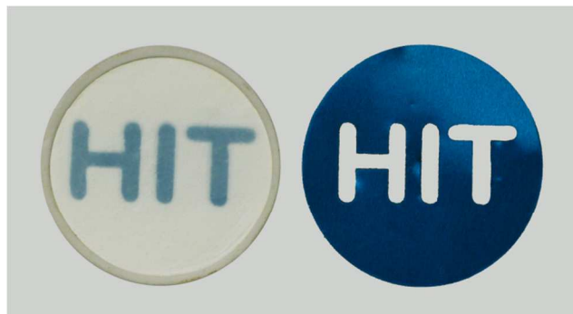
Fig. 6 Visual appearance of the \text{P}_{1100} powders (left image) illuminated through the mask (right image).
