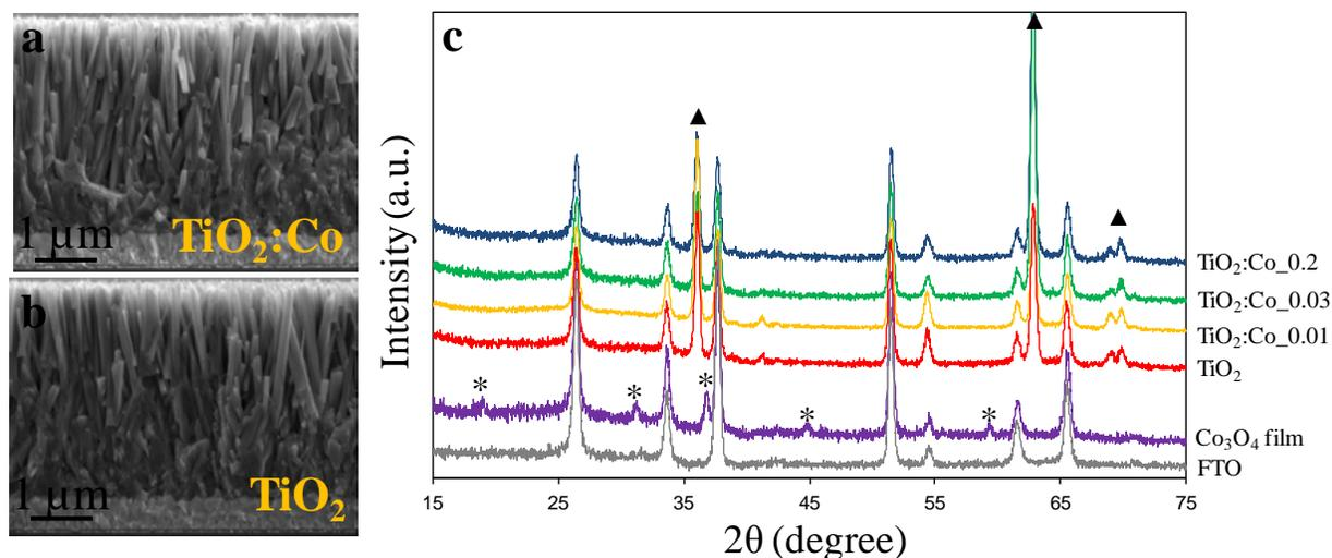
Figure 2. Cross-sectional SEM images of (a) TiO<sub>2</sub>:Co NWs prepared with 0.03 M Co precursor solution and (b) undoped TiO<sub>2</sub> NWs. (c) XRD spectra of TiO<sub>2</sub>:Co<sub>x</sub> ( $x = 0.01, 0.03$  and  $0.2$ ) NWs, undoped TiO<sub>2</sub> NWs, reference Co<sub>3</sub>O<sub>4</sub> film and FTO substrate. Symbols ▲ and \* indicate peaks of rutile TiO<sub>2</sub> phase and cubic Co<sub>3</sub>O<sub>4</sub> phase, respectively.
