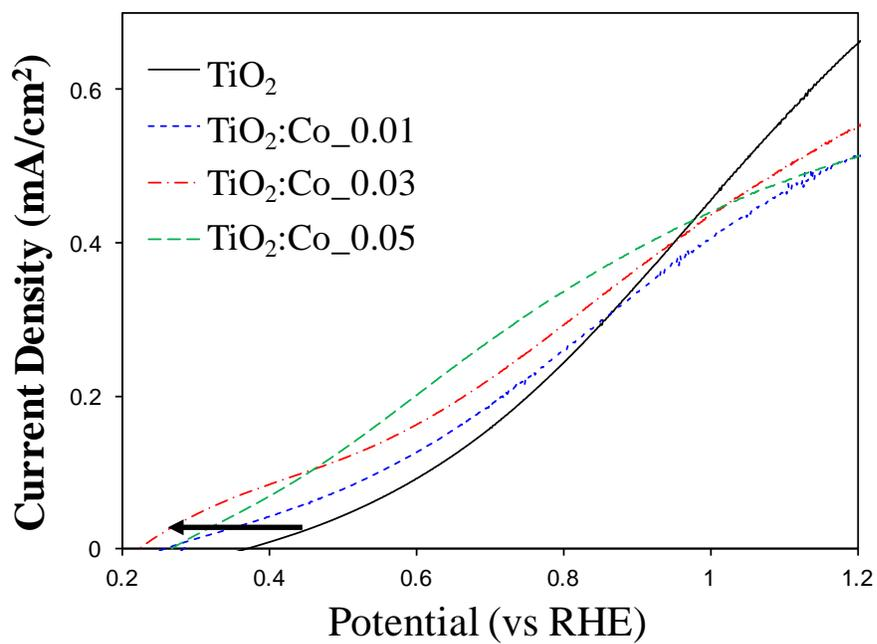
Figure 6. Photocurrent density-potential (J-V) curves of undoped TiO<sub>2</sub> and TiO<sub>2</sub>:Co<sub>x</sub> (x = 0.01 – 0.05) NWs.
