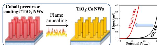
Controllable doping of TiO<sub>2</sub> nanowires with cobalt using sol-flame method, which achieves significantly enhanced electrocatalytic activity for oxygen evolution reactions.
