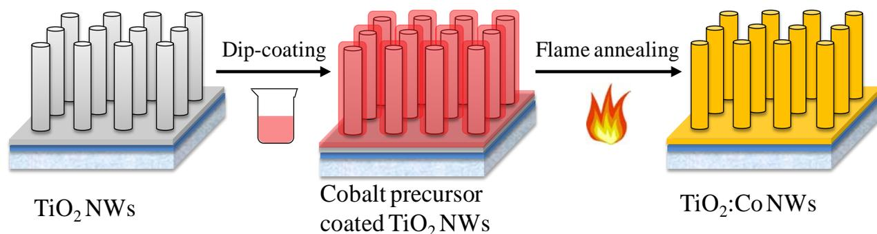
Figure 1. Schematic of the sol-flame doping method for synthesizing TiO<sub>2</sub>:Co NWs.
