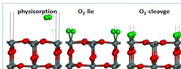
Stage-6: O<sub>2</sub> adsorption on SnO<sub>2-x</sub>-two O-vac and its recovery
