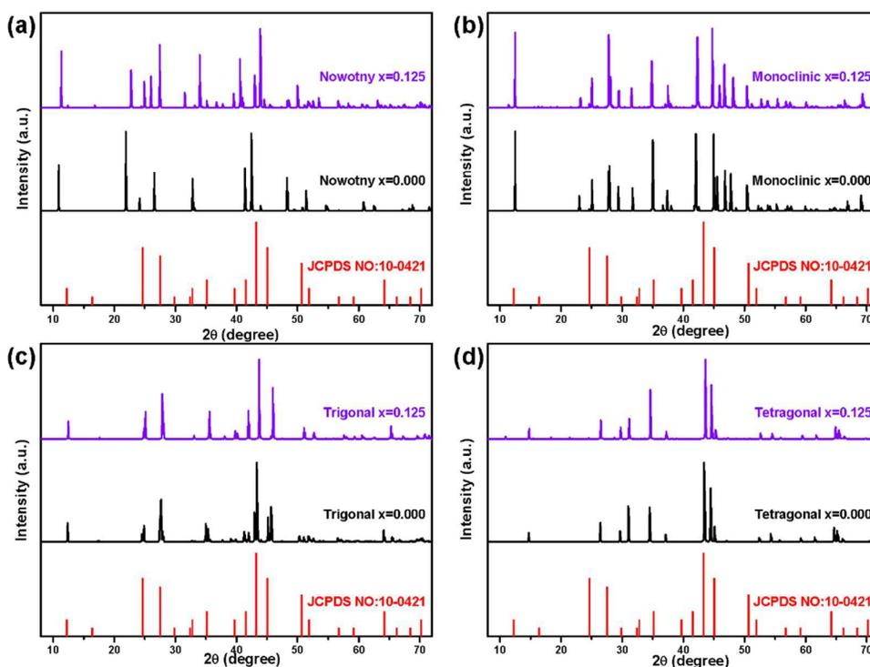
Figure 6. The simulated XRD spectra of  $\text{Cu}_{2-x}\text{Te}$  ( $x=0$  and  $0.125$ ) in (a) Nowotny, (b) monoclinic, (c) trigonal and (d) tetragonal structures. The nominal x-ray source is  $\text{Cu K}\alpha$  ( $\lambda = 0.15406$  nm). The experimental JCPDS peaks are also plotted for comparison.
