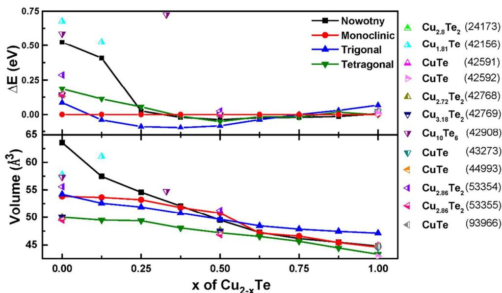
Figure 3. The calculated change of (a) the energy difference between the Nowotny (trigonal and tetragonal) and monoclinic structures, (b) the volume of  $\text{Cu}_{2-x}\text{Te}$  in different structures as a function of  $x$ .
