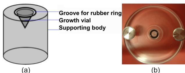
**Fig. 2** (a) A Schematic diagram of the growth cell; (b) The mounting plate with an inserted growth cell.
