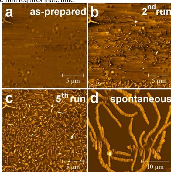
Figure 2: Phenytoin thin film with 15 nm thickness after the preparation process (a), the 2<sup>nd</sup> AFM scan (b), the 5<sup>th</sup> AFM scan induced (c) and the spontaneously formed crystals.
