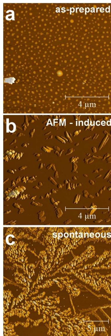
Figure 1: Phenytoin thin film with a sub monolayer coverage after the preparation process (a), after the AFM induced crystallization (b) and the spontaneously formed crystals.
