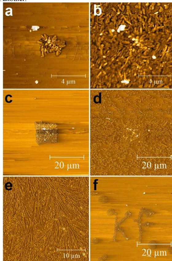
Figure 3: First (a) and 5<sup>th</sup> (b) AFM height image scan of a 50 nm thick phenytoin film. The first (c) and 5<sup>th</sup> (d) scan of the same sample at larger scan ranges. Spontaneously formed (e) and lithographically (f) written crystalline phenytoin surfaces.
