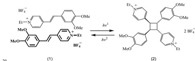
**Scheme 11.** Direct and back PCA reactions in single crystal **1d**.
