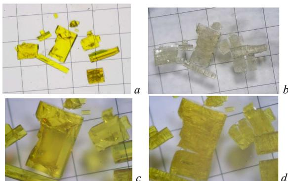
**Figure 13.** Crystals of **1d** in perfluorinated oil on a glass support with 2D millimeter scale: *a* and *c* before irradiation; *b* and *d* after irradiation with unfiltered light of Fiber Optical Light Source (200 W, Meiji Techno) during 10 min (*d*) and 2 h (*b*). Photographs are made using a EMZ-13RT microscope (Meiji Techno).
