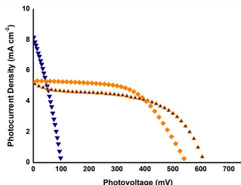
Figure 2. Current-voltage plots for a CAD3/NiO p-DSC (triangles), D35/TiO<sub>2</sub> n-DSC (diamonds) and a D35/CAD3 p/n DSC (open triangles).
