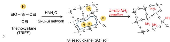
Fig. 1 Schematic image of controlling the pore size and the affinities of TRIES-derived membranes via an *in-situ* reaction between  $\text{NH}_3$  and Si-H groups.
