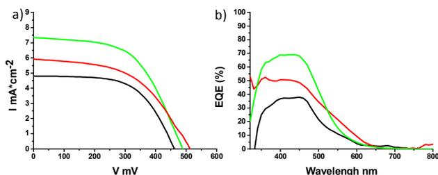
**Fig. 4** (a) J/V curve of QDSC device (b) IPCE of device. Black line CdSe ref, red line CdS with DMF and green line QD CdS-ZnPc.
