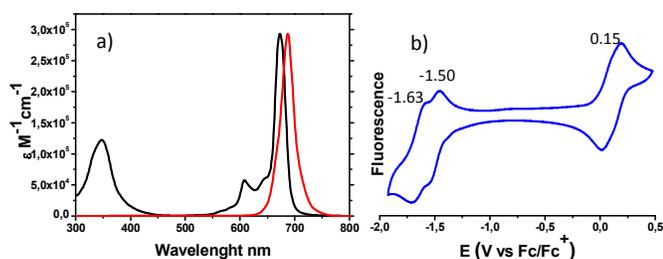
**Fig. 1** (a) UV-Vis and fluorescence spectra of (**(ZnPcS)<sub>2</sub> 1**) in DMF as solvent. (b) Cyclic voltammogram (100 mV s<sup>-1</sup>) of 0.5 mM (**(ZnPcS)<sub>2</sub> 1**) in benzonitrile as solvent containing 0.10 M of TBAPF<sub>6</sub> as a supporting electrolyte.
