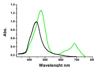
**Fig. 5** Absorbance measurements of QD CdS ref black line, QD CdS-(ZnPcS)<sub>2</sub> green line.
