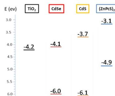
**Fig. 2** Energy levels of TiO<sub>2</sub>, CdSe, CdS and (**(ZnPcS)<sub>2</sub> 1**).
