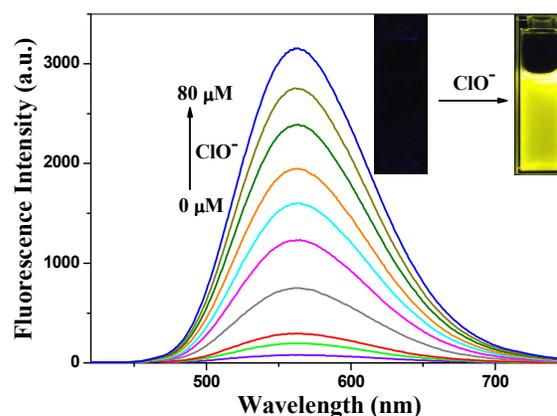
**Fig. 2** Fluorescence titration spectra of PZ-Py (5  $\mu\text{M}$ ) upon addition of NaClO (0, 5, 10, 20, 30, 40, 50, 60, 70, 80  $\mu\text{M}$ ) in PBS (pH 7.3, 10 mM, containing 0.05% DMSO) upon excitation at 400 nm.
