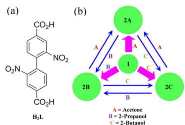
Scheme 1 (a) Structure of ligand H 2 L. (b) Irreversible SCSC transformations between 1 and 2 (A, B, C), and reversible SCSC transformations among 2A , 2B and 2C .
