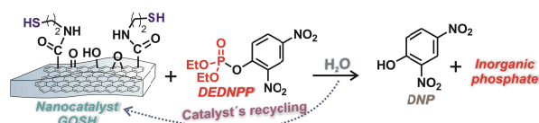
Fig. 1. Reaction of DEDNPP with the nanocatalyst GOSH.
