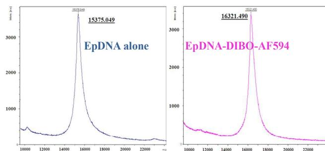
**Figure 3.** MALDI-ToF analysis of the aptamer alone (left panel) and EpDNA-DIBO-AF594 purified from HPLC (right panel) (mass observed were underlined)
