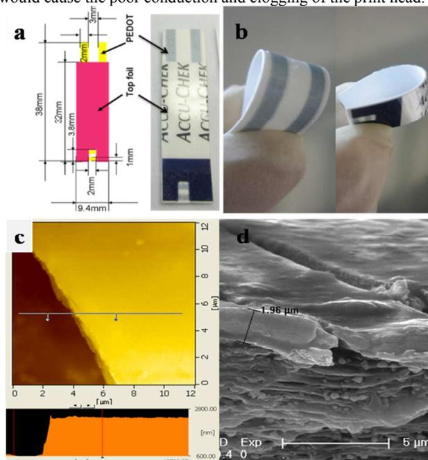
70 Figure 1. Architecture of the flexible MECs and morphology of the electrode. a) The size and pattern of the fabrication of MECs integrated using computer. b) The optical picture of flexible MECs unit on flexible substrates based on inkjet printing technology. c, d) AFM and SEM images of PEDOT:PSS obtained from inkjet printing.
