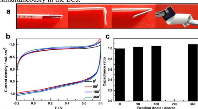
Figure 2. a) Optical images of PEDOT:PSS film bended with different angles. b) Cycle voltammetry of MECs at different bending angles. Scan rate:  $0.08 \text{ V s}^{-1}$ . c) Capacitance ratio of MECs with different angles.
