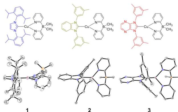
**Figure 1.** Molecular structures (top) and perspective view at 50% probability (bottom) of complexes **1–3**. Only one of the unique structures for **2** found in the unit cell is shown. Hydrogen atoms are omitted for clarity.
