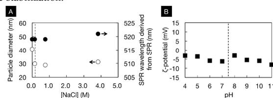
**Figure 2** Colloidal stability of the PMPC-*b*-PMAT-protected AuNPs under (A) high salt concentration and (B) over a wide pH range. The dashed line represents physiological ionic condition. Size of AuNPs for (A) was estimated by dynamic light scattering measurement.
