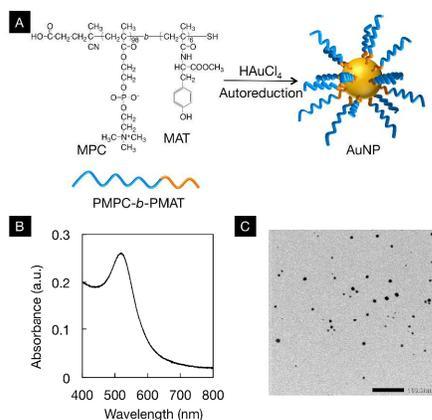
**Figure 1** Synthesis of the PMPC-*b*-PMAT-protected AuNPs: (A) Synthetic scheme of the AuNPs; (B) UV-Vis absorption spectrum of PMPC-*b*-PMAT-protected AuNPs; (C) TEM image of PMPC-*b*-PMAT-protected AuNPs; for (B) and (C), AuNPs was prepared by 3 mM PMPC-*b*-PMAT and each analysis was conducted using AuNPs /153 mM NaCl aqueous solution.
