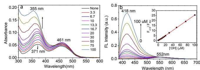
Fig. 3 Changes in the (a) absorbance and (b) fluorescence spectra of 10  $\mu$ M **1** in H<sub>2</sub>O–DMF (98:2, v/v) with the addition of different concentrations of hydroxyl radicals (from 0 to 10 eq). The inset of (b) shows the ratio of emission intensities ( $F_{418}/F_{552}$ ) as a function of concentrations of hydroxyl radicals
