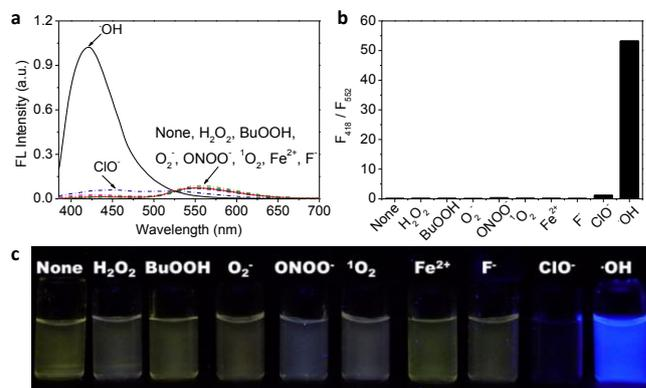
Fig. 2 Fluorescent spectra (a) and images (c) of **1** (10  $\mu$ M) with addition of 50 eq of various ROS in H<sub>2</sub>O–DMF (98:2, v/v,  $\lambda_{\text{ex}} = 365$  nm). (b) The ratio ( $F_{418}/F_{552}$ ) of emission intensities at 418 to 552 nm of **1** with 50 eq of various ROS
