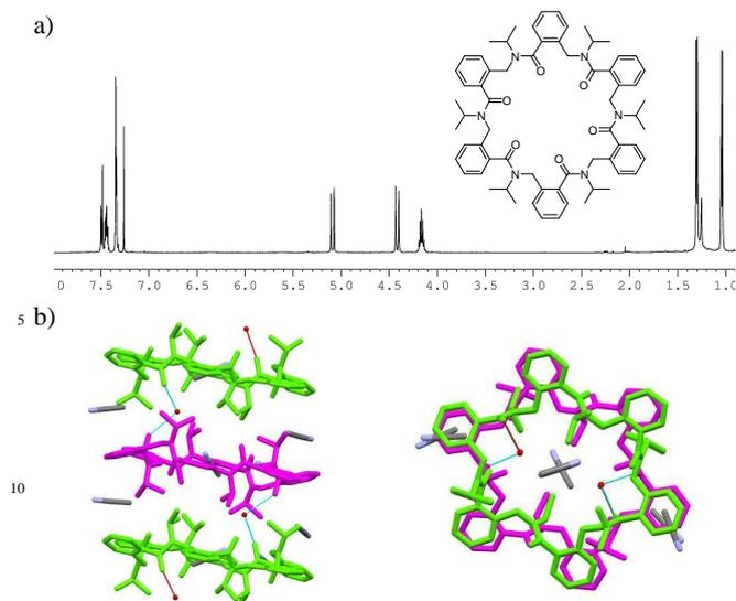
**Fig. 4** a)  $^1\text{H}$  NMR spectra (5 mM in  $\text{CDCl}_3$  at 298K) and structure of **o-3b**; b) Crystal packing of **o-3b**: (left) side view (right) top view (H-atoms omitted for clarity); solvent molecules (acetonitrile) are represented in grey-blue sticks and water molecules as red balls, hydrogen bonding between water and backbone carbonyl groups are highlighted in turquoise blue.
