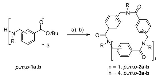
**Scheme 1** Synthesis of macrocyclic arylopeptoids. Key: (a) TFA/CH<sub>2</sub>Cl<sub>2</sub> 1:1, 0 °C, 3 h (*p/m*-**1a-b**) or 0 °C, 3 h and rt, 1 h (*o*-**1a-b**). (b) HATU (1.2 equiv.), DIPEA (approx. 5.0 equiv.), CH<sub>2</sub>Cl<sub>2</sub>/DMF 4:1, 0 °C to rt, 3 d. See Table 1 for yields.
