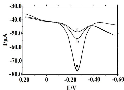
Fig. 6. Differential pulse voltammograms of MB at ssDNA/CS/TiO<sub>2</sub>/ERGO/CILE (a), hybridized with PCR product of *tth* gene sequence (b) and CS/TiO<sub>2</sub>/ERGO/CILE (c).
