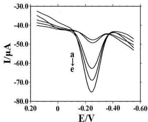
Fig. 4. Differential pulse voltammograms of 2.0×10<sup>-5</sup> mol L<sup>-1</sup> MB after hybridization with 1.0×10<sup>-6</sup> mol L<sup>-1</sup> the target ssDNA sequence (a), noncomplementary ssDNA sequence (b), one-base mismatched ssDNA sequence (c), three-base mismatched ssDNA sequence (d) and at the probe ssDNA modified electrode (e).
