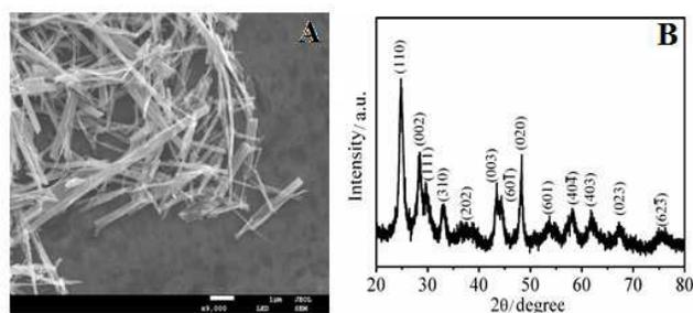
Fig. 1 SEM image (A) and XRD pattern (B) from as-prepared TiO<sub>2</sub> nanowire.
