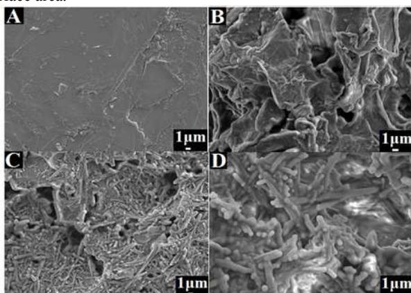
Fig. 2. SEM images of CILE (A), ERGO/CILE (B), TiO<sub>2</sub>/ERGO/CILE (C) and CS/TiO<sub>2</sub>/ERGO/CILE(D).
