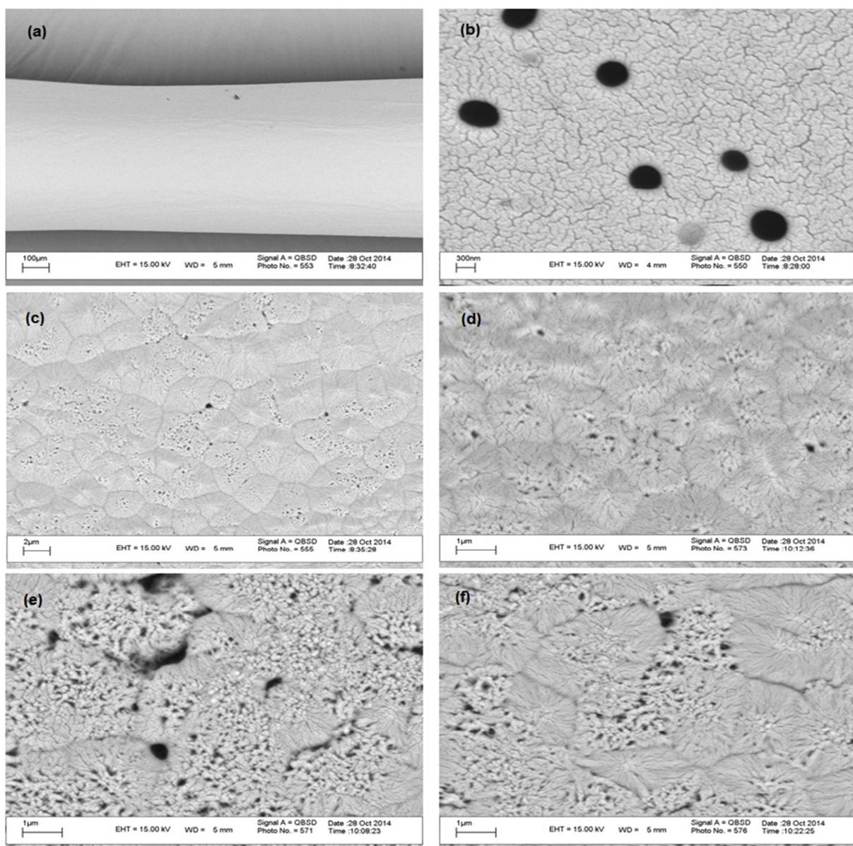
Fig. 2. SEM image of (a) prepared stir bar with the coating of CNTs/PA with CNT doping level of 1 mg (b) bulk PA, (c, d) CNTs/PA with CNT doping level of 1 mg, (e) CNTs/PA with CNT doping level of 10 mg and (f) CNTs/PA with CNT doping level of 15 mg.
