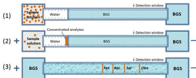
**Fig.2** Schematic diagram of a preconcentration mechanism with FESI. (1) Pressurized injection of water plug; (2) Field-enhanced sample injection; (3) Separation after injection.
