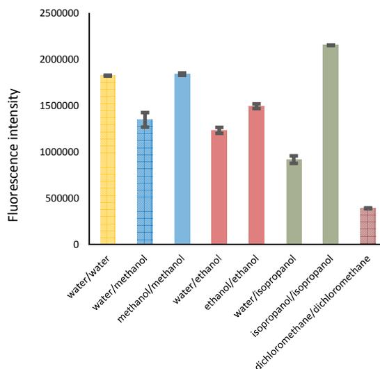
Figure 2: Fluorescence intensity and standard deviation of QS measured in combination of different solvents - effect of the carrier stream/acidified QS solution composition
