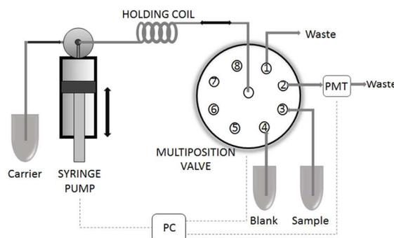
Figure 1: Set-up of the sequential injection system
