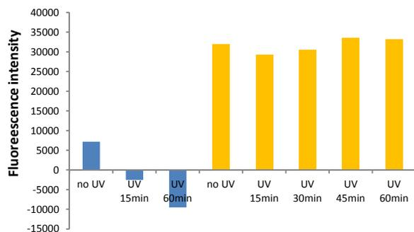
Figure 4: Fluorescence intensity of MSM in the mixture of water and acetonitrile (ratio of 7 : 3) - blue (without pH adjustment), yellow (pH 2)
