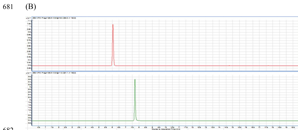
683 Fig. 4. Example of a HPLC-MS/MS chromatogram of a standard mixture at 100 \mu\text{g} 684 \text{L}^{-1} for target compounds analyzed by (A) positive ion mode and (B) negative ion 685 mode.
