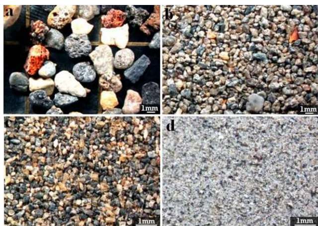
Fig.2 Microphotographs of the obtained particle sizes: a) <2 mm, b) 250 \mu\text{m} - 2mm, c) 75-250 \mu\text{m} and d) < 75 \mu\text{m} .
