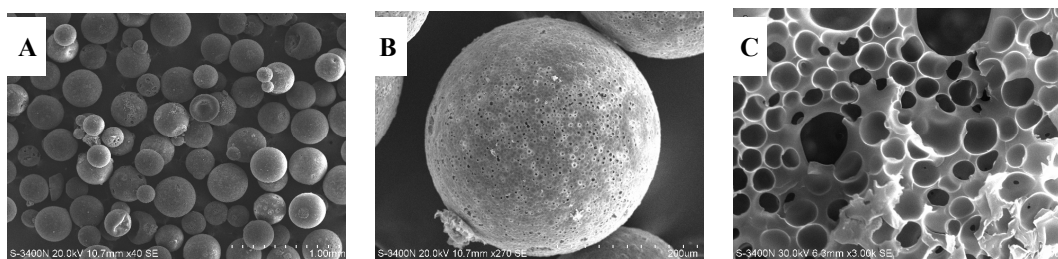
Fig.4. SEM images of MIP at (A) \times 40 , (B) \times 270 , and (C) \times 3000 showing the presence of pores
