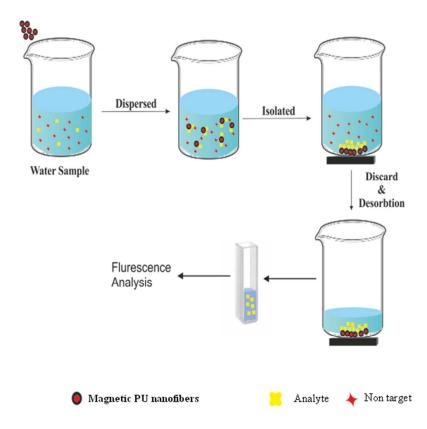
The extraction/desorption setup for isolation of fluoxetine. 187x158mm (96 x 96 DPI)
