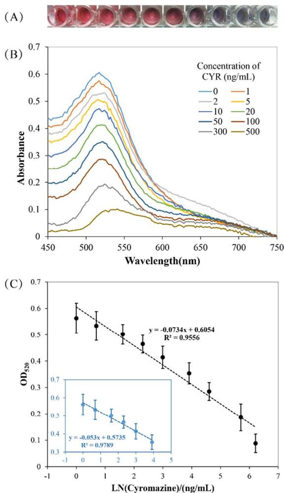
**Fig. 3** Sensitivity and linearity of the polyT10-AuNP based colorimetric assay for CYR detection. (A) Visual color changes of AuNPs in the water solution containing different concentrations of CYR. (B) The UV-vis absorbance spectra changes of AuNPs. (C) The absorbance value changes of 520 nm in linear with the logarithm of the CYR concentrations in the range from 1 ng/mL to 500 ng/mL. Inset: from 1 ng/mL to 50 ng/mL.
