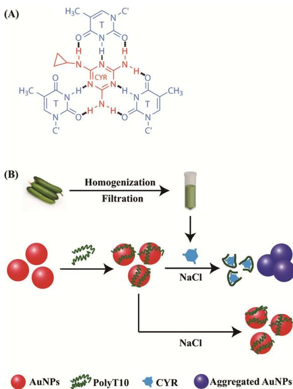
**Scheme 1.** (A) The structure of the hydrogen-bonding recognition between CYR and thymine. (B) The working principle of CYR detection. Label-free AuNP sensor for optical analysis of CYR.
